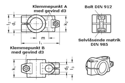
Adjustable clamp lever for  $d3 = GN \ 911-M10-55$  have to be ordred separately Adjustable clamp lever for  $d4 = GN \ 911-M \ 8-32$  have to be ordred separately d1 = 42 d2 = 25 d3 = M10  $d4 = M \ 8$  d4 = 65 d5 = 59
